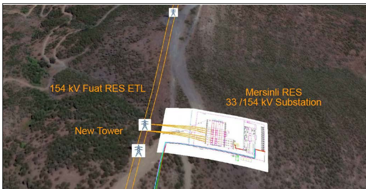
Figure 3–2. Mersinli WPP Project Substation and ETL Connection
