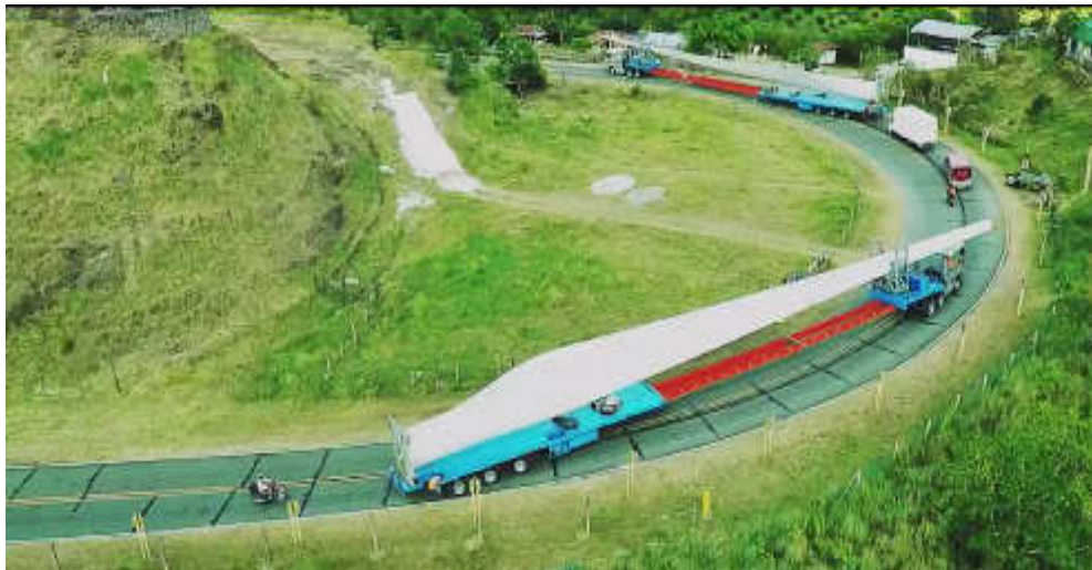
Figure 4-5 Typical Special Trucks For Transporting Propeller Blades
