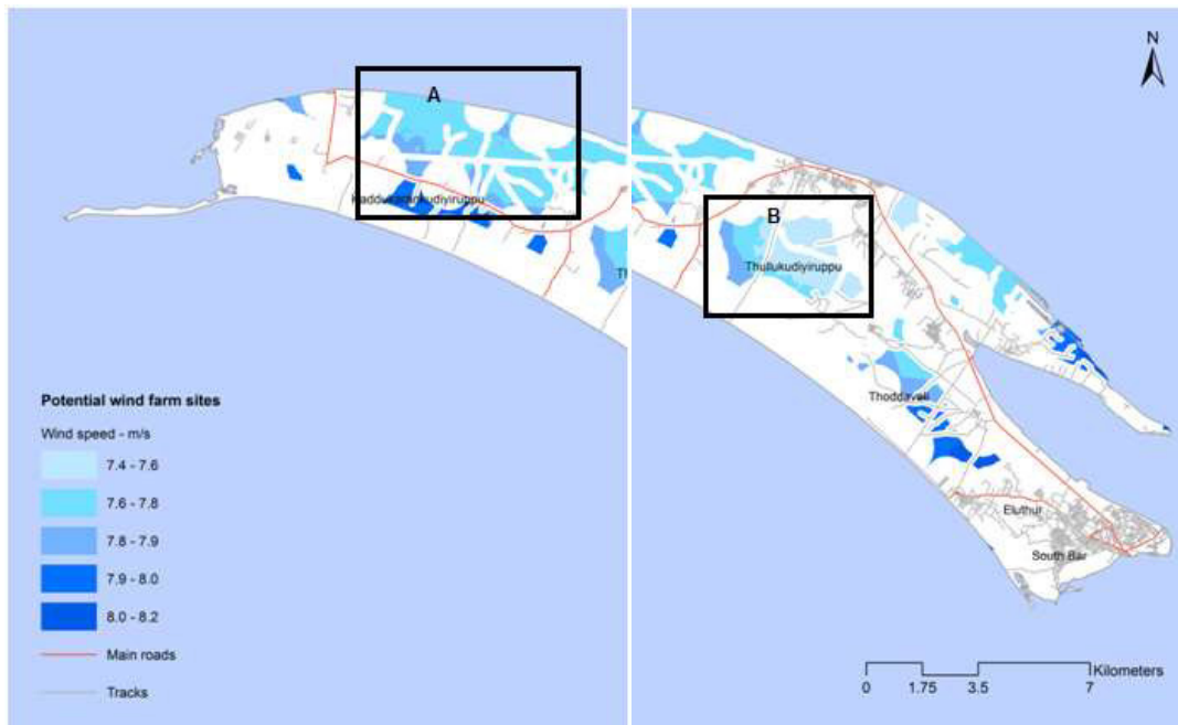
Figure 3.2: Areas potentially available sites for future wind farm development in the Mannar Island (only blue areas inside the rectangles A & B)
