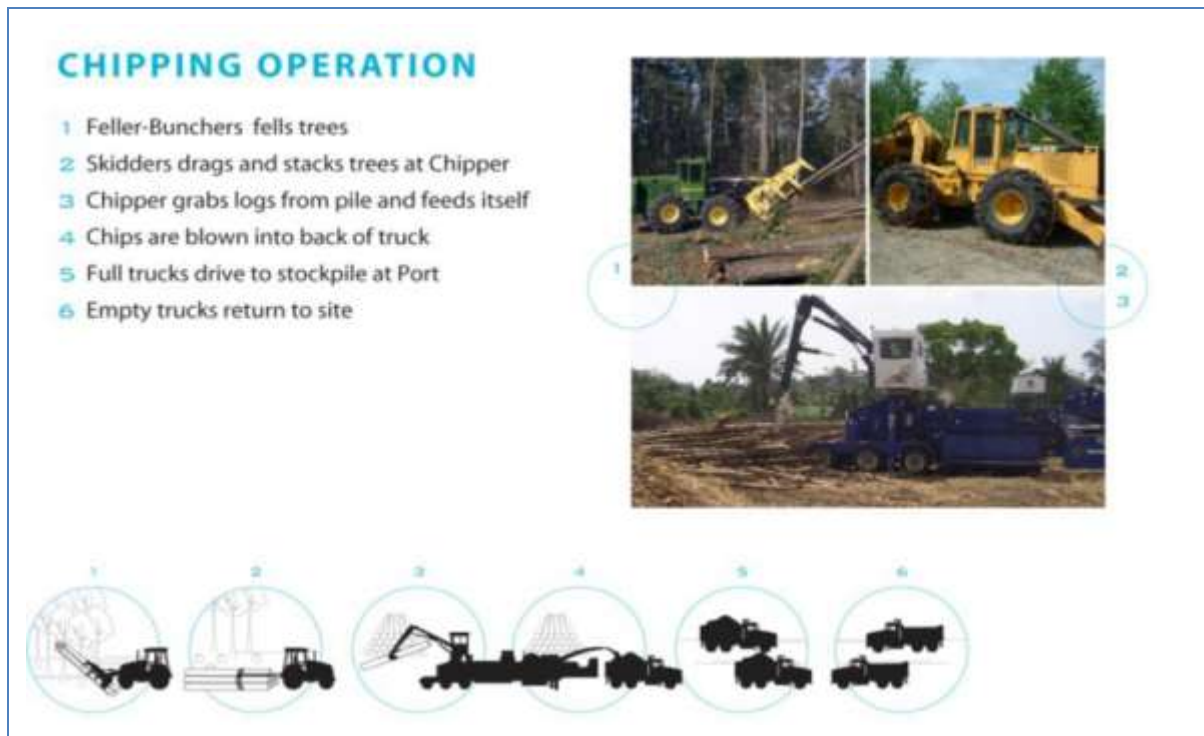
Figure 4-3: Stages of chipping operations. Source: Buchanan Renewables Fuel.
