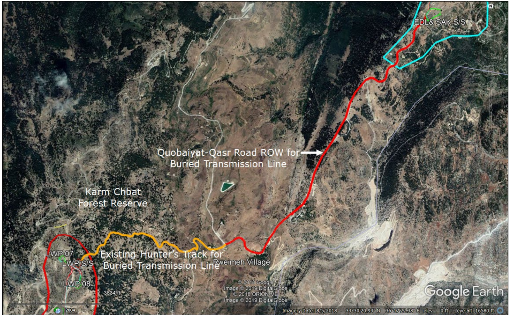
Figure 2-5 Alignment of Buried Transmission Line
