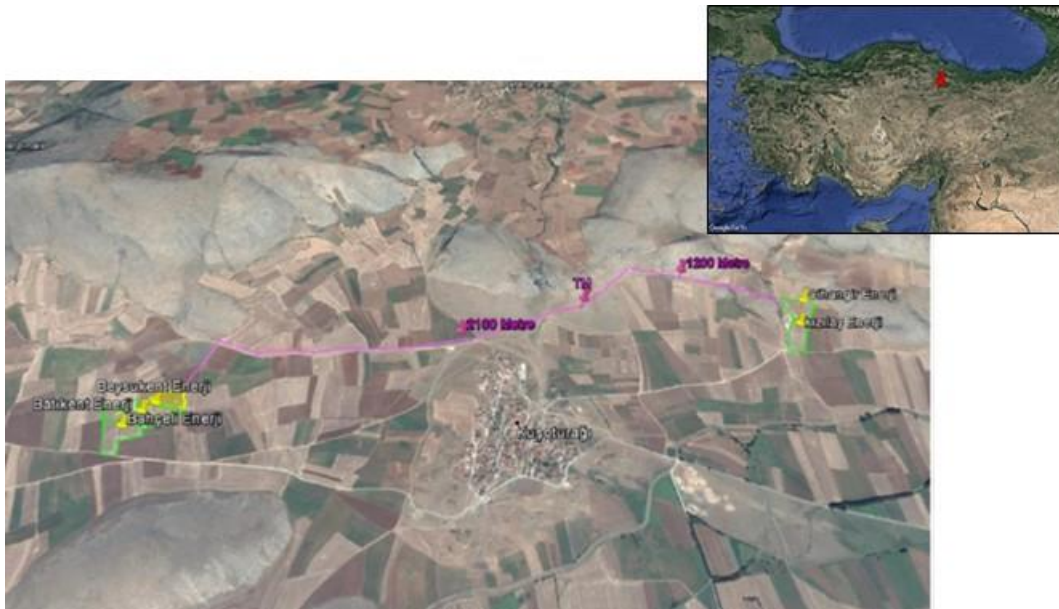
Figure 1: A satellite view of the Tokat Solar Power Plant sites near Kuşoturağı village (in green) and the transmission line (in purple)
