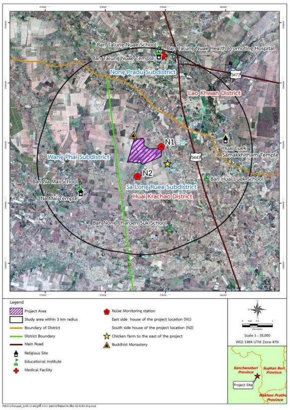
FIGURE 4.2.1-1: NOISE MONITORING STATIONS AND SENSITIVE RECEPTORS
