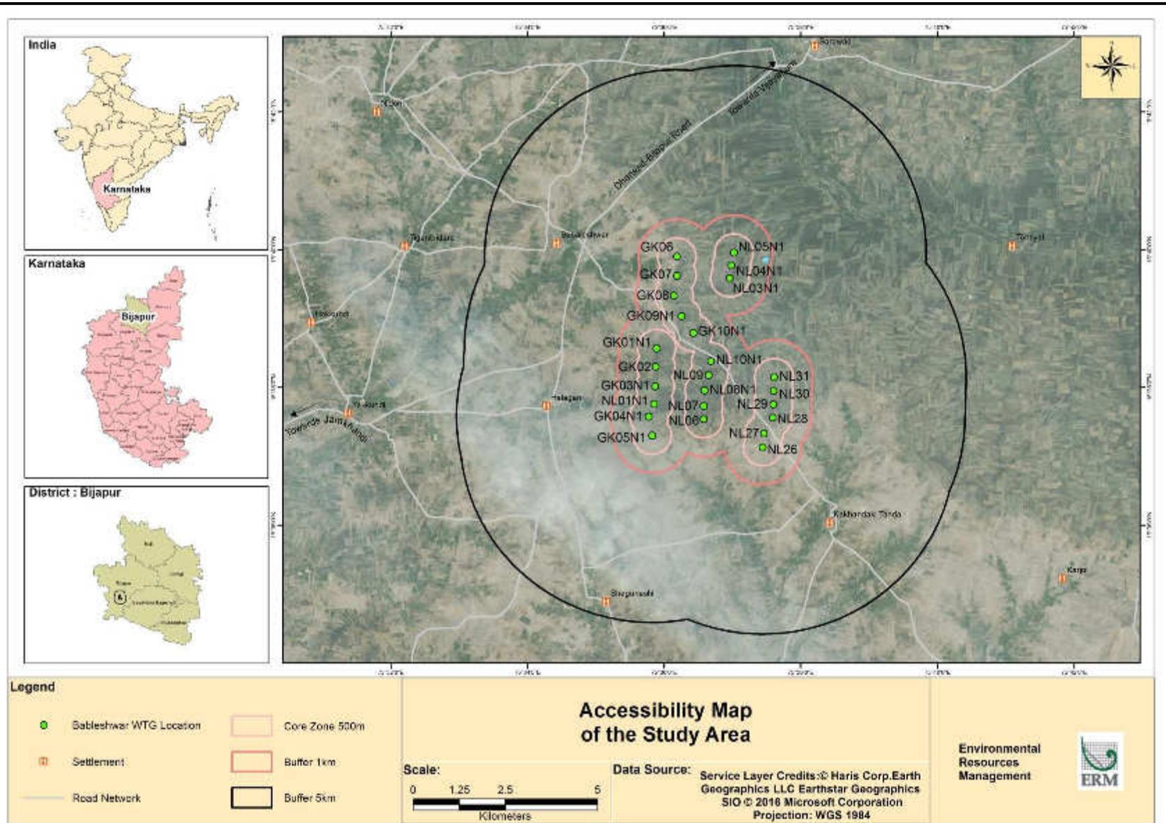
Access to the wind farm is through 8 m width village roads that connect Halagani, Bableshwar and Khandaki Tanda Villages. Access to individual WTGs has been created by constructing roads of approximately 8 m width and a turning radius of 45 m.
