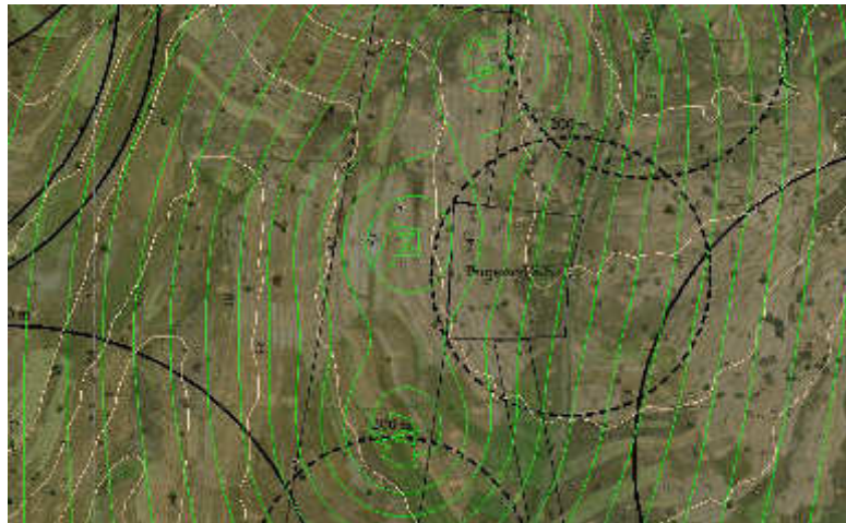
7. Use optimized layout to undertake noise impact analysis and overlay results on high resolution imagery
