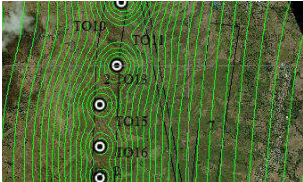
Noise assessment output represented by green contours using DNV GL's WindFarmer for analysis
