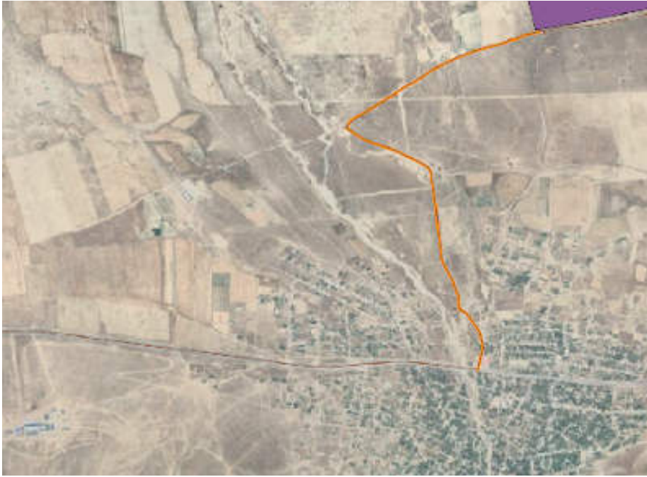
Figure 23: Access Road 5320 m. Orange line – access road, brown line – track 5.04.2024, violet polygon – Nurabad substation (March 2024).
