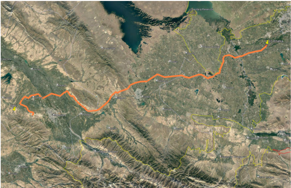
Figure 3: Khalka substation and 360 km 550 kV OHTL
