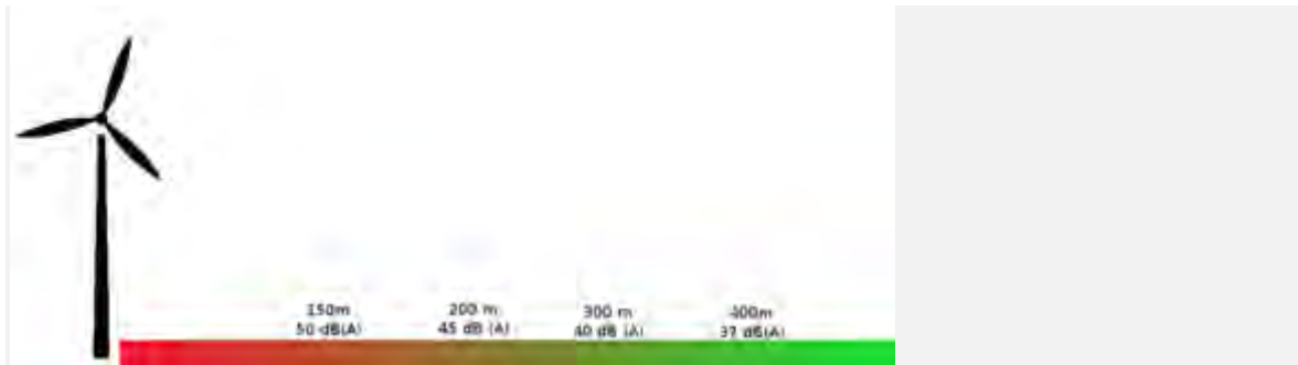
Figure 46: Mitigation of the noise according to the distance away from the wind turbine
