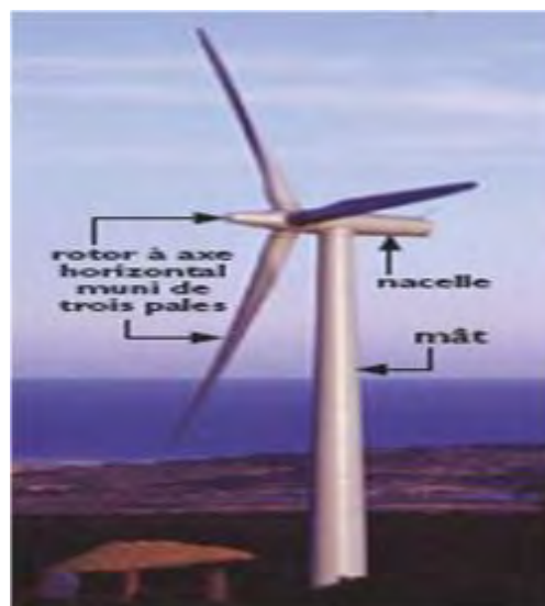
Rotor with a horizontal shaft fitted with three blades
