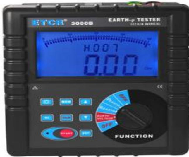
The maximum depth of the probe did not exceed 20cm nor exceed 1/20<sup>TH</sup> of the probe spacing distance 'a'. A series of resistivity readings are taken for various spacing of the probes. For this site the spacing increased to enable the soil resistivity to be assessed at a greater depth.
