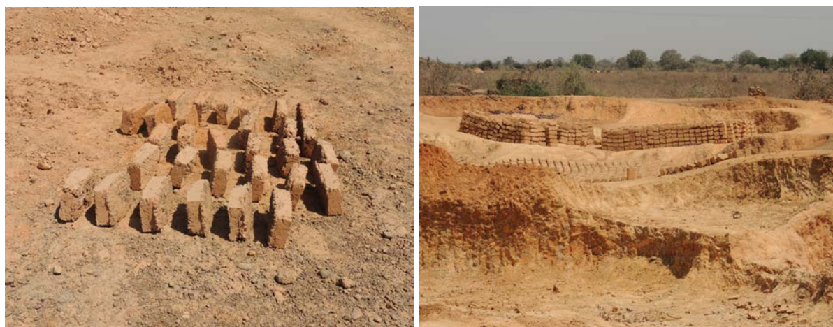
Figure 4.25: Laterite Mined at the Project Site and Used for Block-Making
