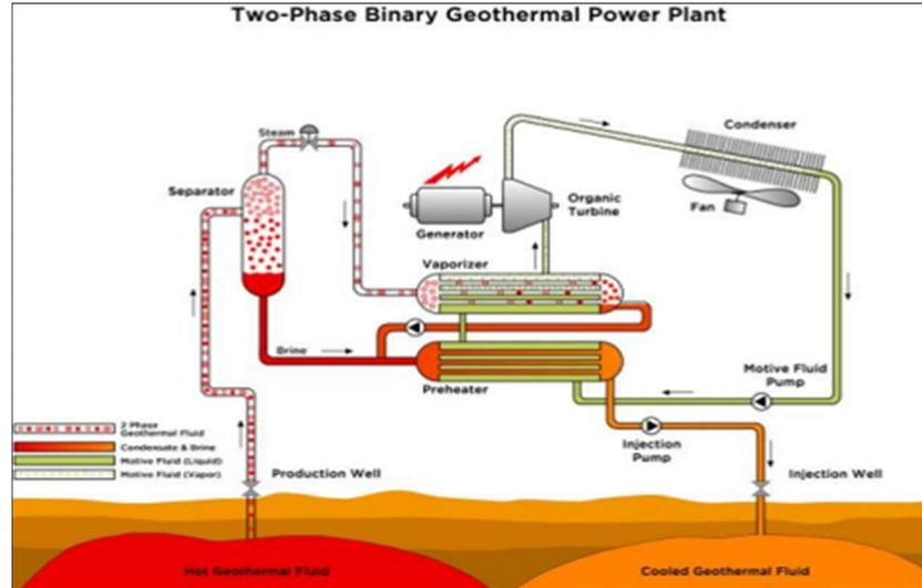
Figure of Two phase Binary Geothermal Power Plant
