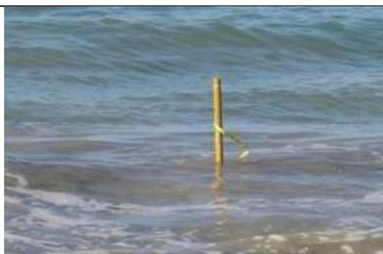
**Figure 4.36: Temporary tide staff for recording water level changes**
