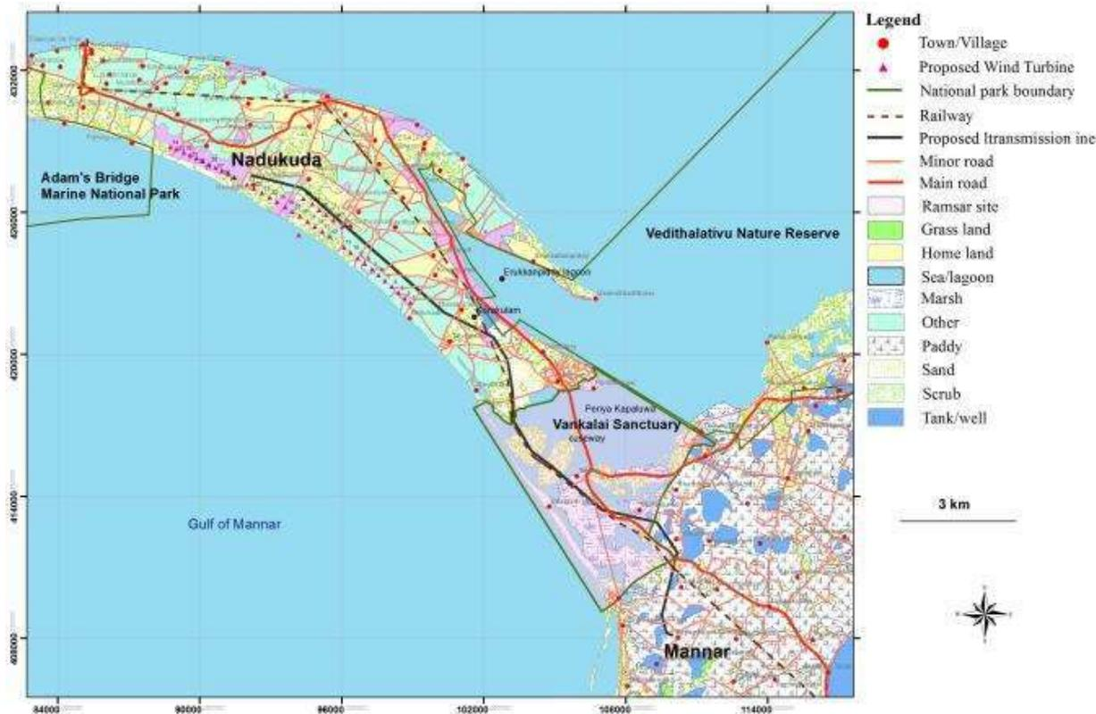
**Figure 3.8: Wind turbines location in respect to three important bird areas**
