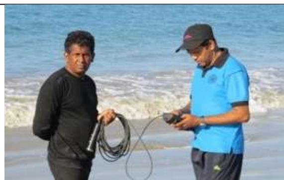
**Figure 4.35: Multiparameter reader (YSi Pro Plus) used to measure, temperature, DO, TDS, EC, salinity and pH**
