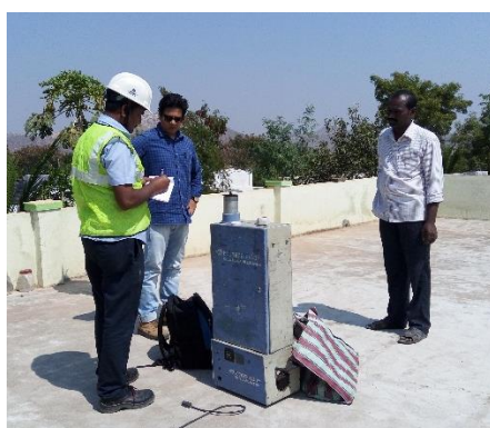
Air Quality Monitoring at Veligallu
