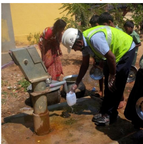
Ground Water Collection from Thumu kunta Village
